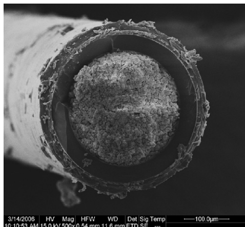
Figure 2. SEM of the monolith completely filling a 250 \mu\text{m} capillary.
